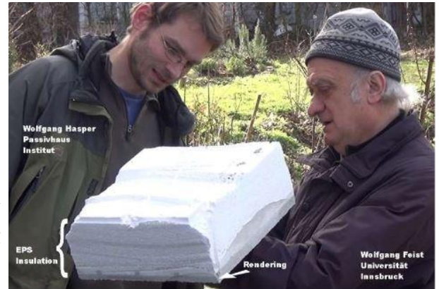
Perfect state: Wolfgang Feist (right) and a colleague examine the insulation of the first Passive House. The piece was removed from the wall of the building on the occasion of the 25th anniversary of its completion. © PHI
