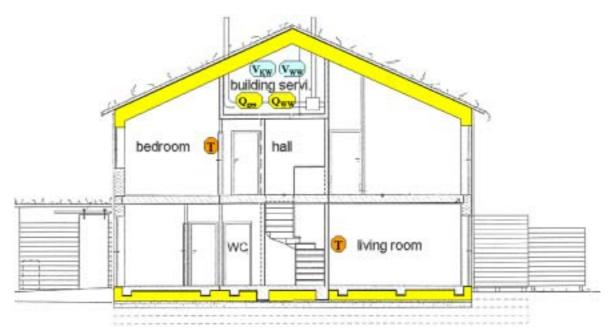
Figure 39: Cut-away section through a terraced Passive House with drawn-in location of the measurement points for the standard measurement (according to [Pfluger 2000]).
