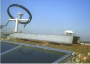
Figure 43 and Figure 44: Weather station in the Passive House estate. <u>Left</u>: Telescope pole with the sensors. <u>Right</u>: Radiation measurement units with and without shadow ring on the ridge.
